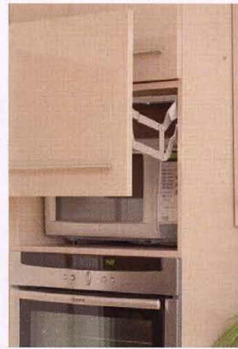
MICROWAVE CUPBOARD To save space on the worktop, the microwave sits in a unit above the oven. The door pulls out and up for easy access
